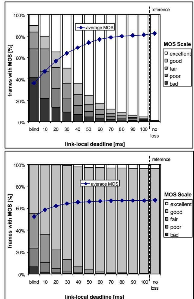
Figure 4 MOS of video transmissions with blind and fixed-deadline scheduling (top: high-motion video, bottom: low-motion video)
