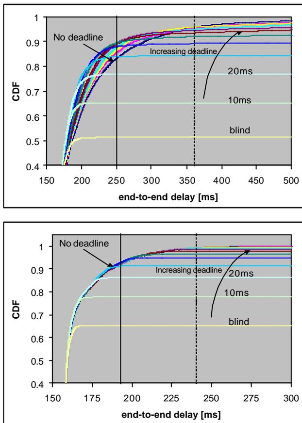
**Figure 5 Cumulative Distribution Function (CDF) of the video frame end-to-end delays (top: high motion, bottom: low motion)**
