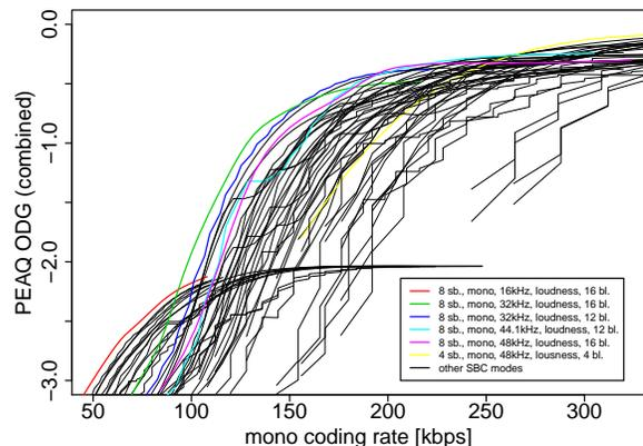
Figure 1. Using SBC for mono audio
