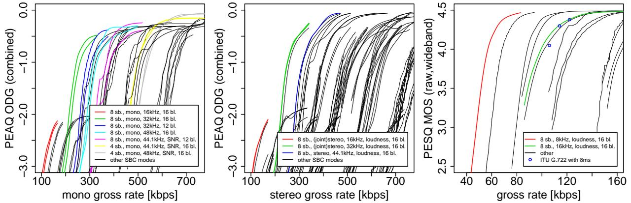
Figure 2. Using SBC for mono audio, stereo audio, and speech measuring the gross rate (including RTP, UDP, IPv4, and Ethernet packet headers)
