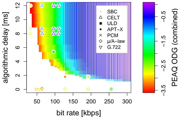
Figure 3. Objectively audio quality measured with combined PEAQ of samples encoded with different codecs and different coding modes. We display the ODG value versus algorithmic delay and bit/gross rate.
